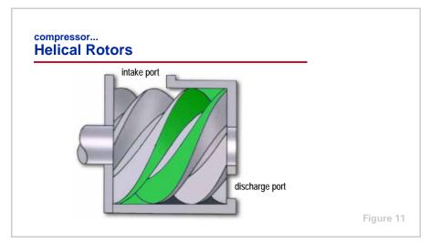
Viewing the compressor from the side shows that after the pockets of refrigerant travel to the right past the intake port area, the vapor, still at suction pressure, is confined within the pockets by the compressor housing.
